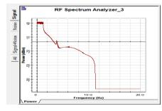
Figure4. Filtered OFDM signal by LP filter
