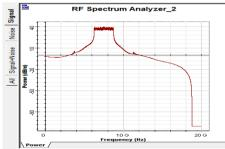
Figure 5. OFDM Signal in the Frequency Domain
