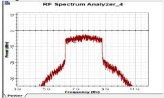
Figure8. RF Signal after BPF
