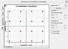
Figure3. 16 QAM Encoder Constellation Diagram
