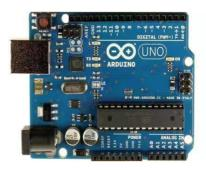
The Arduino Uno is a microcontroller board based on the ATmega328. It has 20 digital input/output pins (of which 6 can be used as PWM outputs and 6 can be used as analog inputs), a 16 MHz resonator, a USB connection, a power jack, an in-circuit system programming (ICSP) header, an reset button. It contains everything needed to support the microcontroller; simply connect it to a computer with a USB cable or power it with a AC-to-DC adapter or battery to get started.
