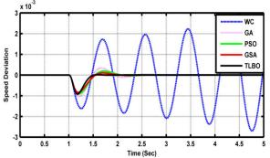
Fig.13 Speed Deviation for 25% Increase in Direct Axis Time Constant at (b) condition
