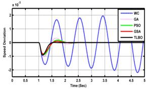
Fig.14 Speed Deviation for 25% Decrease in Direct Fig.15 Speed Deviation for 25% Decrease in Direct Axis Time Constant at (a) condition
