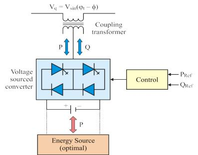
Fig.2: Transmission line with SSSC.
