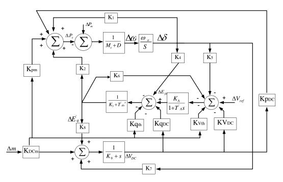
Fig.4 Haffron Model of SMIB with SSSC [7]
