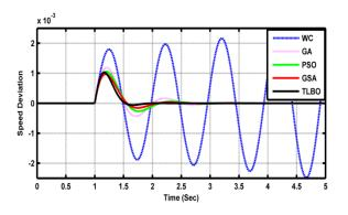
Fig.8 Speed Deviation for 25% Increase in Machine Inertia at (a) condition
