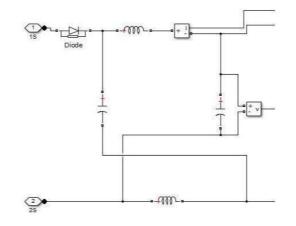
In Above Fig. it consists of split inductor L1 and L2 and capacitors C1 and C2 connected in X shape. These two L and C is employed to provide impedance source(Z-source) coupling with the converter (or inverter) to the load. Therefore, dc source can be a battery, fuel cell, diode rectifier or any dc fed supply, we have proposed the dc source can be a battery. The inductance L1 and L2 can be provided through a split inductor or two separate inductors.
