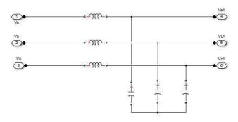
The Above Fig. shows that second order filter used in the Z-source inverter. This filter circuit has been used to filter the harmonics in the dc equivalent voltage before applied to the bridge inverter.
