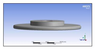
Figure 2: CAD model of disk brake
