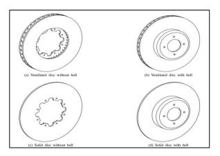
Figure 1: Types of disk brakes
