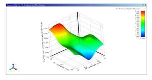
Figure 17: 3D response surface plot of directional heat flux
