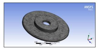
Figure 3: Meshed model of disk brake
