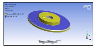
Figure 4: Loads and boundary conditions
