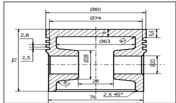
Figure 2: Schematic of piston [7]
