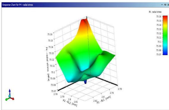
Figure 14: Response surface plot of radial stress in horizontal direction
