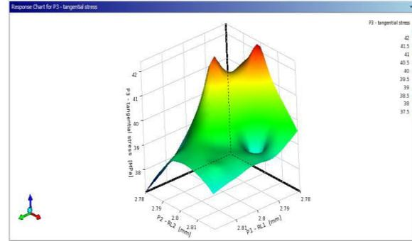
11: Response surface plot of tangential stress in vertical direction
