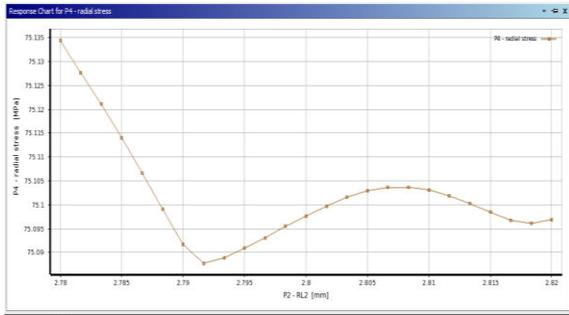
Figure 13: Radial stress vs ring land 2 (RL2)
