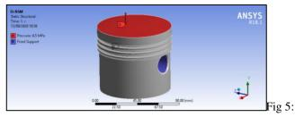
Applied structural loads and boundary conditions
