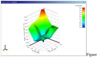
14: Response surface plot of radial stress in horizontal direction
