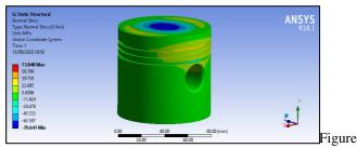
6: Radial stress distribution on piston using Eutectic alloy
