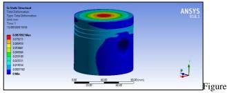
8: Deformation plot on piston using Eutectic alloy
