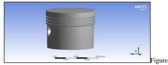
3: Imported CAD model of piston in ANSYS software
