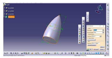
Fig.6 CAD model of Nose Cone
