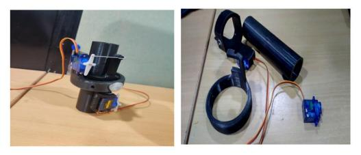
Fig.8. 3D printing of Assembled TVC
