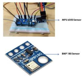
or D The MPU6050 is a Micro Electro-Mechanical Systems (MEMS) which consists of a 3-axis Accelerometer and 3-axis Gyroscope inside it. This helps us to measure acceleration, velocity, orientation, displacement and many other motion related parameter of a system or object.
