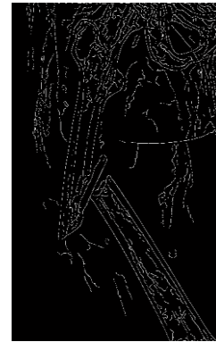
Fig.5. Edge detected image using canny operator
