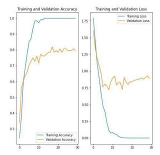
Figure 5:Output of the Training with Overfitting.
