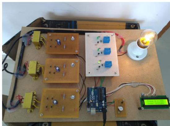
Fig 5: With phase A undervoltage, phase C active
