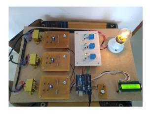
Fig 5:With phase A undervoltage, phase C active
