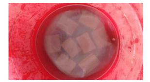
Fig 5.5 water absorption test
