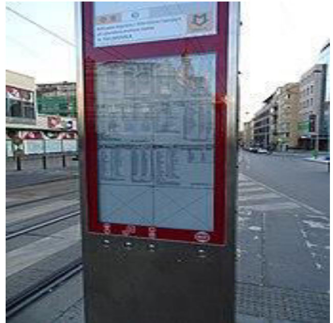
FIGURES - E-PAPER PROTOTYPE OF TRAP TIMETABLES IN PRAGUE, FROM MAY 2009.
