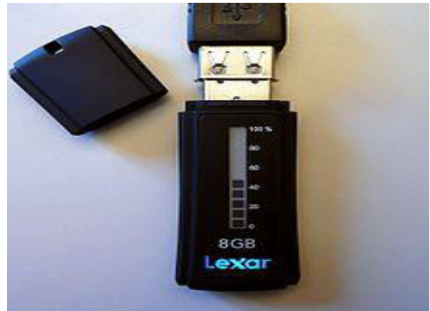
FIGURE3 - A USB PENDRIVE SHOWING THE AVAILABLE STORAGE SPACE USING AN E-INK DISPLAY.
