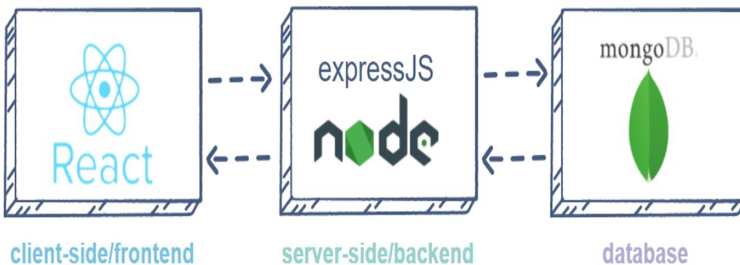
**Figure 3: Working of MERN Stack**
