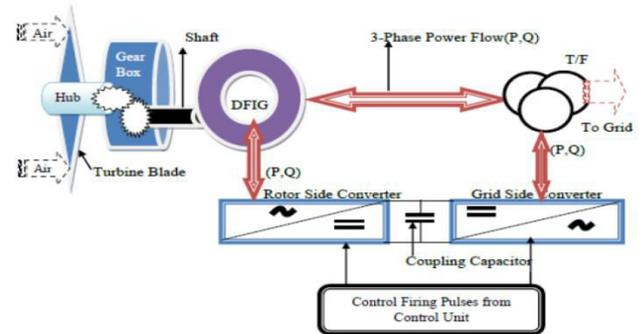
Fig. 1 DFIG with power converter
