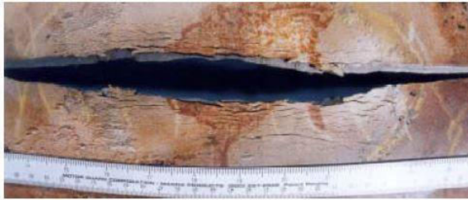
Figure 10 Drill pipe failure, Fatigue
