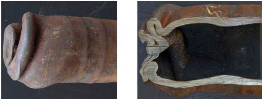
Figure 8 Drill pipe failure, Twist off
