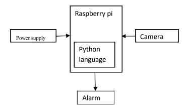
The architecture of the driver drowsiness system has been shown in the above Fig. The camera captures the image and sends to the Raspberry pi which consists of 32 bit memory card installed with Open CV which helps in image processing.
