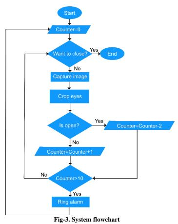
The counter-based method gives better performance than time-based method. But in this method, we have to finetune maximum threshold with respect to system speed.
