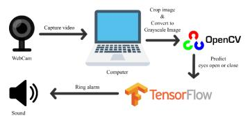
Fig-2. System architecture
