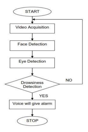
**Fig-1:** Flow-Chart about how system operates
