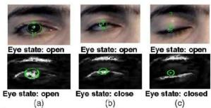
These is a image were it shows the region of interest (ROI). It is a process in which it detects the portion of an image that we want to operate. In our project eyes are relevant to us, only eyes can detect the person is sleepy or not.
