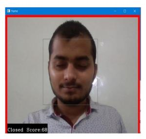
Here, the  $2^{nd}$  image shows the eyes are closed for long time. A certain threshold value is defined if the score is more than 15 eyes are closed for long time. If the eyes get close it will beep an alarm and driver get alert form getting accidents.
