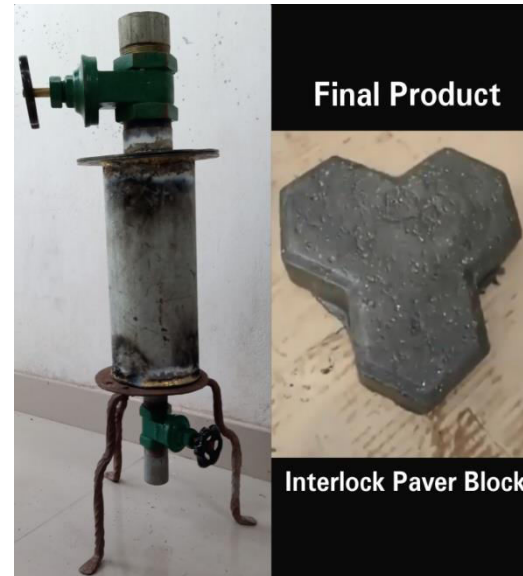
Fig 4.4 Boiler and Final Product
