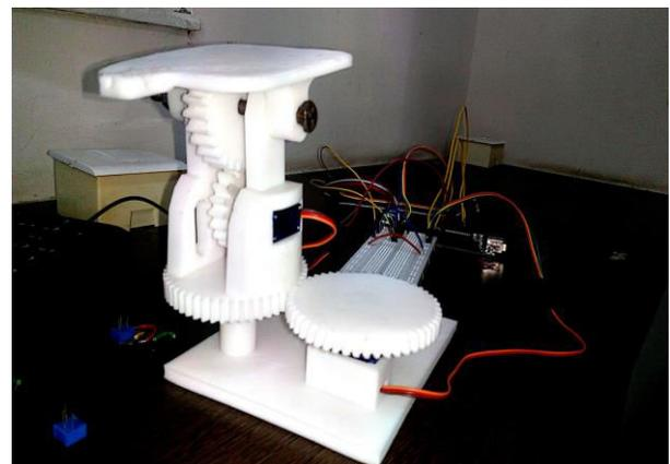
Fig 2: Prototype of Dual-axis solar tracker.
