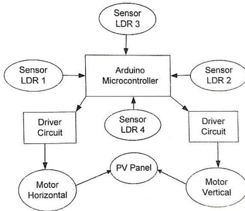
Fig 1: Block diagram of Dual axis solar tracking system.
