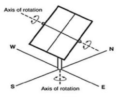
Fig - 4: Two axis Tracking sytem
