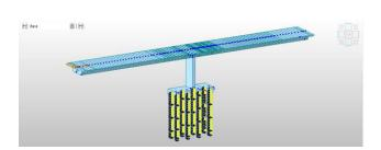
Fig.(6): Elastic spring for pile foundation
