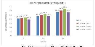
Fig 4 Compression Strength Test Results
