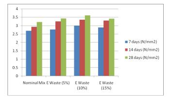
**Fig 7 Flexural Strength Test Results**
