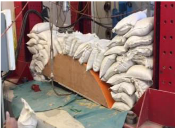
Figure 5: Arched sandbag roof system
