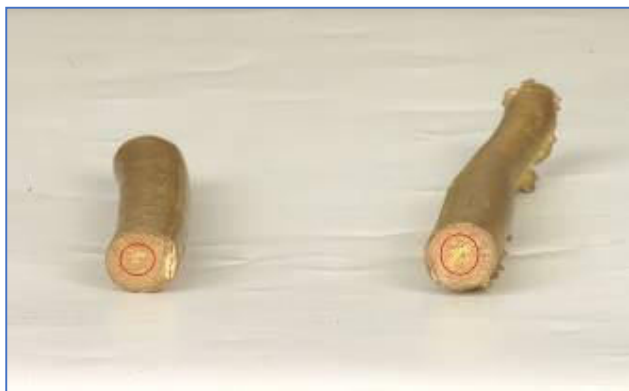
Figure 1: Encircled red shows defect in Brass casting shows coring & Segregation
