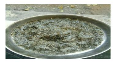
**Figure 1- Chopped Basalt Fibre**
