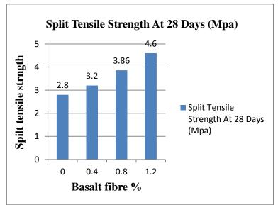
Graph 3 Split Tensile Strength At 28 Days(Mpa)
