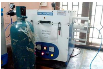
Fig-4: Tubular furnace
