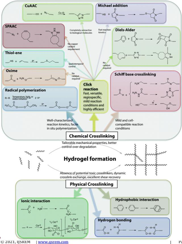
**Fig. 6** Chemical functional groups for hydrogel formation. A wide range of functional groups is available for either hydrogel formation or modification post-polymerization. Functional group selection depends on several factors related to the application of interest, including the desired initiation mechanism, the specificity and speed of the reaction, and the stability of the resulting bond under various solution conditions.
