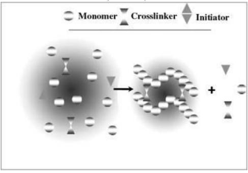
Fig. 24. Schematic diagram of hydrogel preparation.
