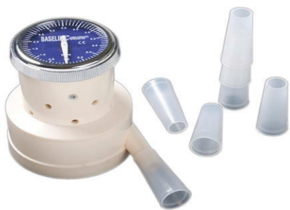
Fig-7: Wind Mill Type Spirometer
