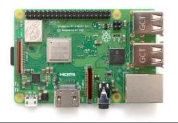
Fig. 3 Raspberry Pi Model 3B+
