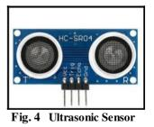
Ultrasonic Sensors operate on the basic principle of using sound waves to determine fluid level. The frequency range for ultrasonic methods is ~20-200 kHz. A transducer directs the sound waves downward and it bursts onto the surface of the water. Echoes of these waves return to the transducer, which performs calculations to convert the distance of wave travel into a measure of height, and therefore water level.
