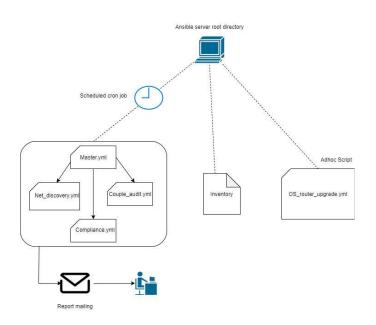
Fig -4: Architecture of ansible server and its functions
