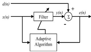
Fig-2.3: Block diagram of Adaptive filter
