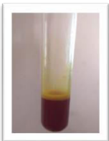
Fig.7 Detection of Alkaloids - Mayer's test
