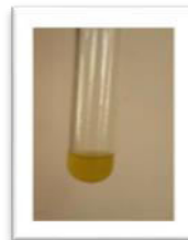
Fig.10 Detection of Terpenoids - Salkowshi's Test
