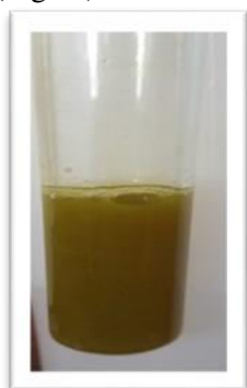
Fig.14 Detection of Proteins - Biuret's Test
