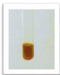
Fig.12 Detection of Steroids - Liebermann-Burchard test
