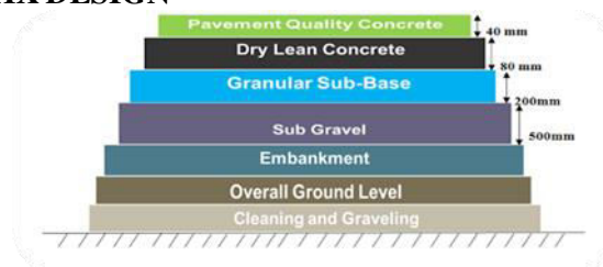
Fig:1 Layers on rigid pavement FOR 1M LENGTH
