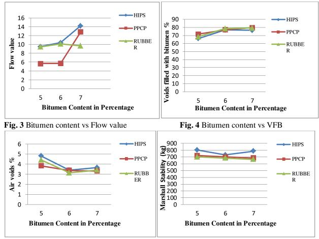
Fig. 5 Bitumen content vs Air voids
