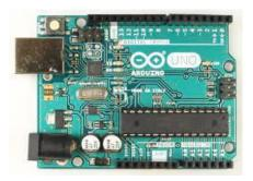
Arduino Uno is a microcontroller board based on 8-bit ATmega328P microcontroller. Along with ATmega328P, it consists other components such as crystal oscillator, serial communication, voltage regulator, etc. to support the microcontroller. Arduino Uno has 14 digital input/output pins (out of which 6 can be used as PWM outputs), 6 analog input pins, a USB connection, A Power barrel jack, an ICSP header and a reset button.
