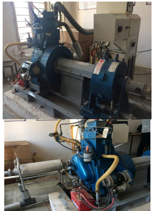
Fig. 3.2 Experimental setup of VCR Diesel Engine
