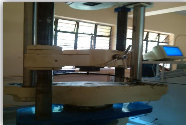
Fig.No.02- Conventional leaf spring under loading Condition
