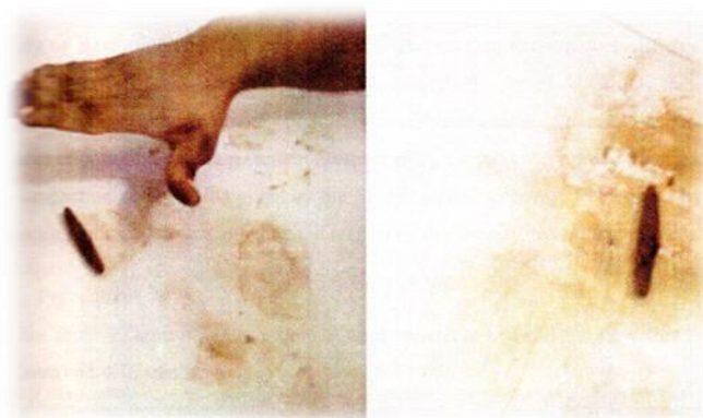
Fig-3 Plastic Limit Test (thread before & after crumble)
