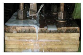
Fig 6.5.Five layers of Carbon fiber polyester bolted to the slotted table milling machine
