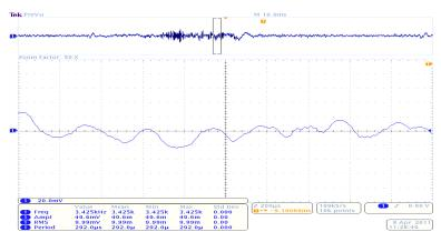
Fig 7.5 Vibration signal for single layer of carbon fiber.
