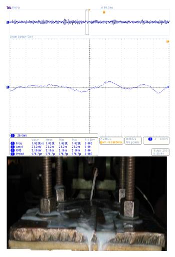
Fig 6.9 one layers of Carbon fiber polyester bolted to the slotted table milling machine
