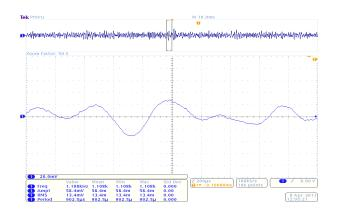
Fig 7.1 Vibration signal for five layers of Carbon fiber polyester plates
