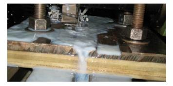
Fig 6.6 Four layers of Carbon fiber polyester bolted to the slotted table milling machine
