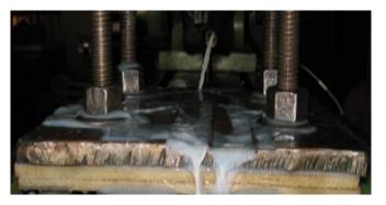
Fig 6.8 Two layers of Carbon fiber polyester bolted to the slotted table milling machine
