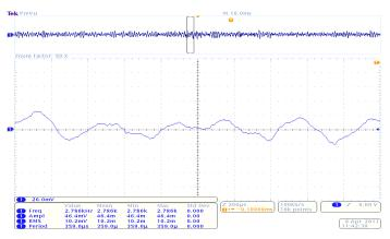
Fig 7.2 Vibration signal for four layers of Carbon fiber polyester plates
