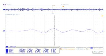
Fig 7.4 Vibration signal for two layers of Carbon fiber polyester plates
