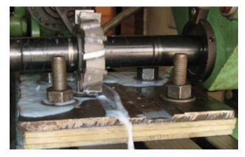
Fig 6.7 Three layers of Carbon fiber polyester bolted to the slotted table milling machine.
