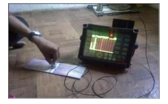
Fig. 5 UT of aluminum welded plate
