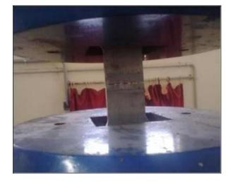
Fig. 10 Arrangement of bending
