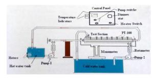
Figure 1 Schematic diagram of experimental Setup
