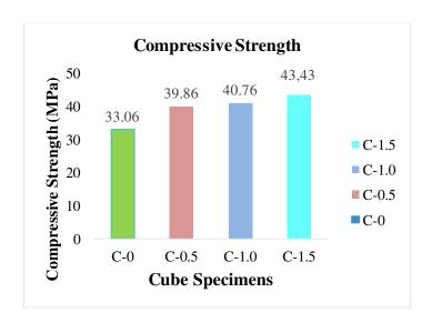
Figure 2: Compressive Strength of GFRC (28 days Curing)
