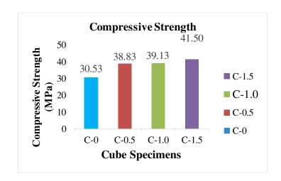
Figure 1: Compressive Strength of GFRC (7 days Curing)
