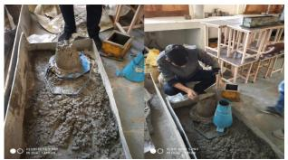
.1 Slump testing by Slump Fig cone apparatus with different percentages of plastic
