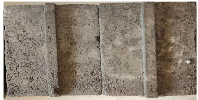
Fig.10 Efflorescence Test
