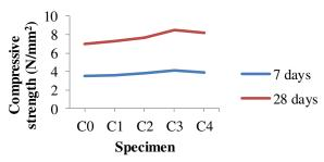
Fig.3 Compressive strength test for specimen C
