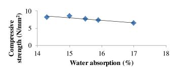
Fig.13 Relationship between compressive strength and Water absorption for specimen C
