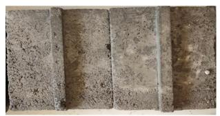
Fig.10 Efflorescence Test
