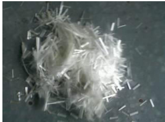
Figure 3.1: glass fibres Strands (12mm) used as a reinforcing concrete
